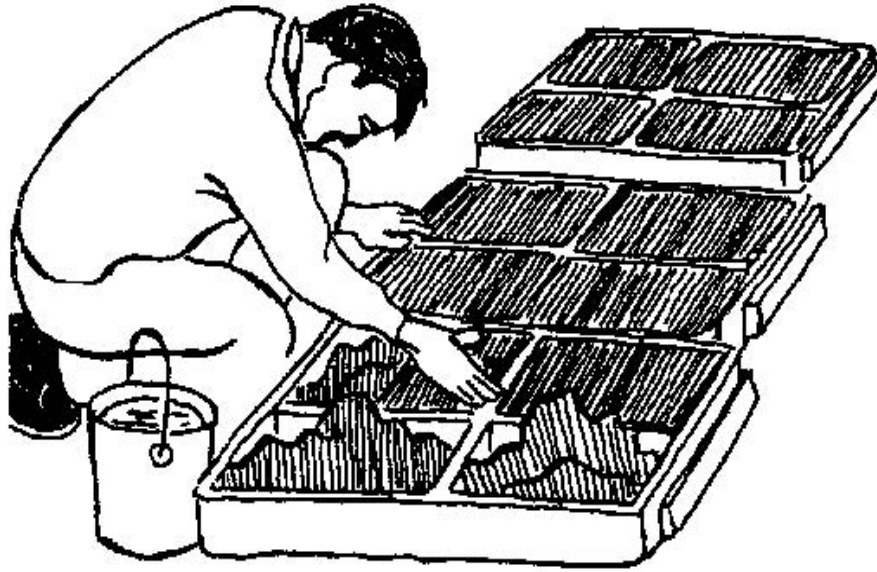
Figure 40. Kneading and leveling the blocks
